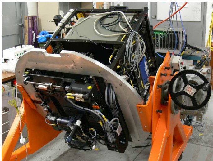
Figure 22. Instrument on its tilting trolley undergoing final tests before shipping to Hawaii. The frame above and to the rear holds the electronics; its enclosure covers are not fitted. The FPI is below and to the front.
